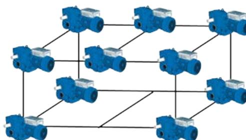
Meshed earthing bands have proved effective for the connection of metal components. Usually, these have cross sections of **10 mm<sup>2</sup> to 25 mm<sup>2</sup>**.
