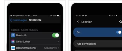
Important information before starting Bluetooth scanning: Turn location on for your mobile device to enable Bluetooth scanning for the NORDAC ACCESS BT on your mobile Android devices. Enable Bluetooth access for the NORDCON APP on your mobile iOS device. Important information in case a Bluetooth connection to the dongle is not possible: The Bluetooth lock
