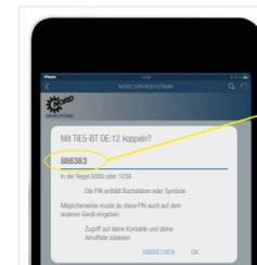
If you are asked for the PIN, type the last 6 digits of the ID number on the type label of the NORDAC ACCESS BT and then couple the devices.
