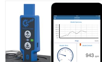
The dashboard opens, and the Status LED lights up blue. The NORDAC ACCESS BT is now connected with the terminal device.
