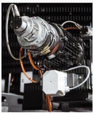
Whisper-quiet technology Thanks to a special counter-bearing concept to reduce noise, the NORD drive units are especially quiet in operation.
