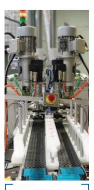
WGC mobile canning lines range from 2 to 4 fill heads and have a 27-42 can per minute filling capacity
