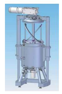
Robust single-piece construction. – Industrial geared motors at the agitator handle massive loads.
