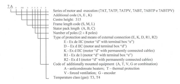
According to the type of protection, ambient temperature range and the model, the motors series 7 A 315 can have the following marking:
