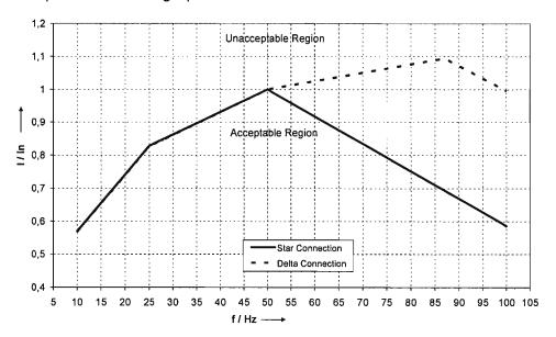
Setting parameters for continuous-current limit of the frequency converter between 10 Hz and 100 Hz
