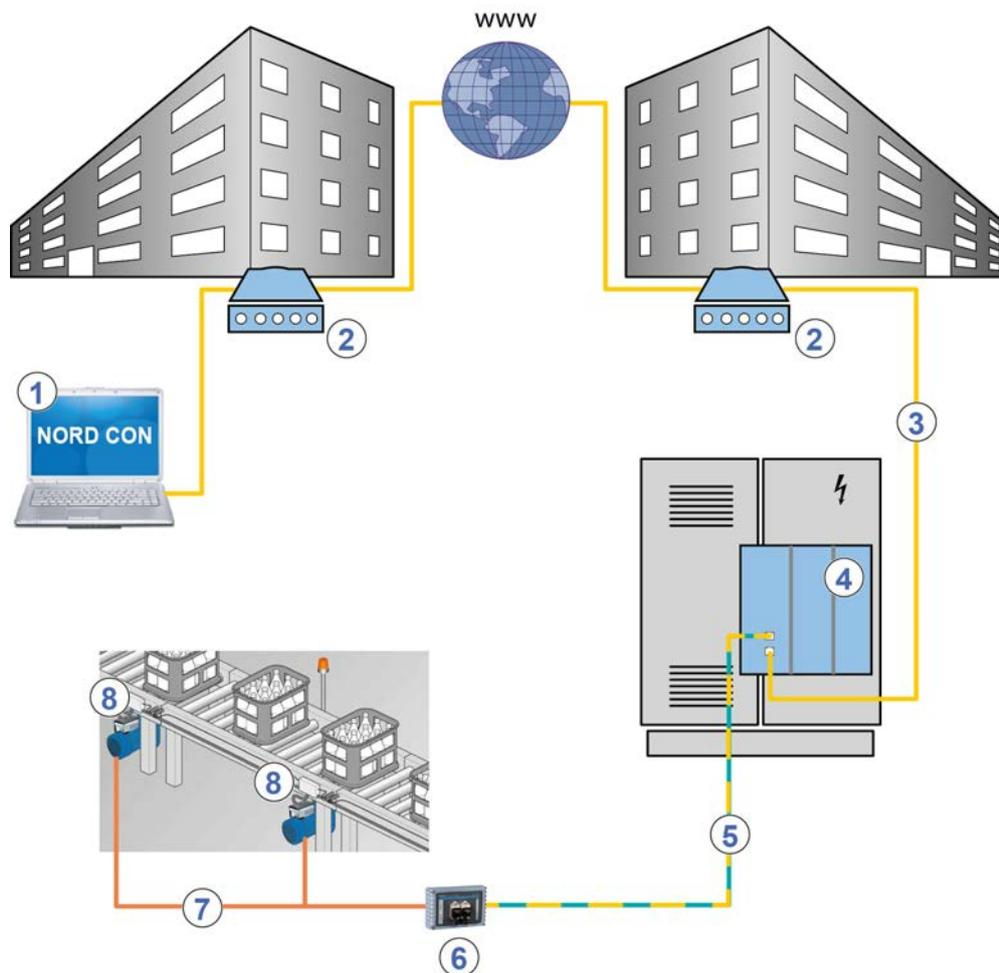
Figure 13: Remote maintenance via Internet (schematic diagram)
