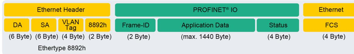
Figure 7: PROFINET IO telegram (communication within a sub-net)
