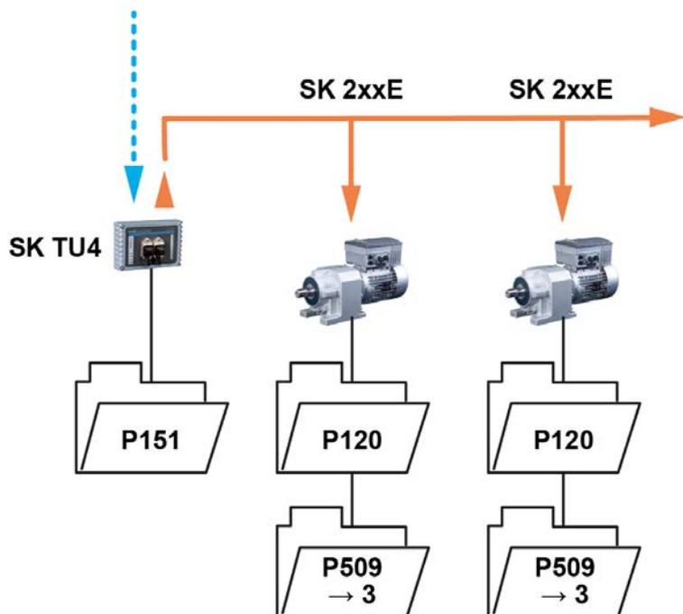
Figure 19: Examples of monitoring parameter settings – SK TU4 bus interface
