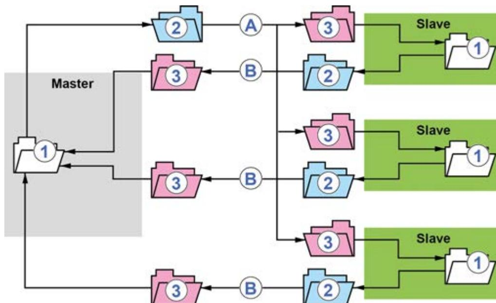
Figure 7: Bit Strobe I/O Connection
