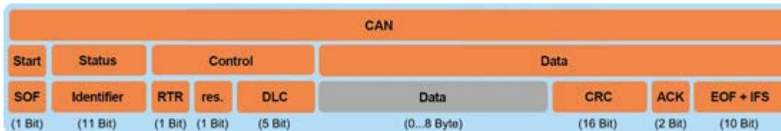
Figure 3: CAN standard frame – 11-bit identifier
