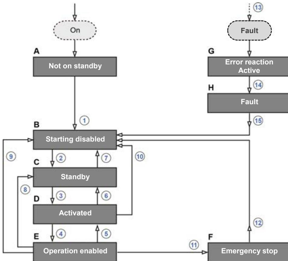
Figure 9: Frequency inverter status machine
