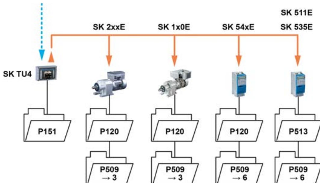
Figure 10: Examples of monitoring parameter settings – SK TU4 bus interface
