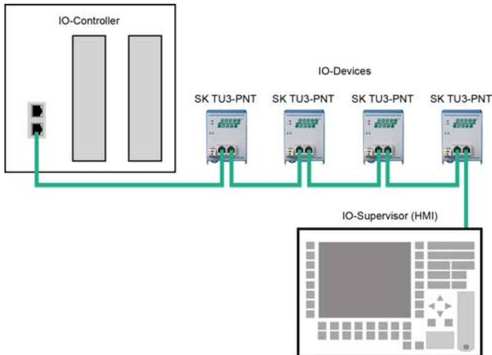
Figure 2: Linear topology (example)
