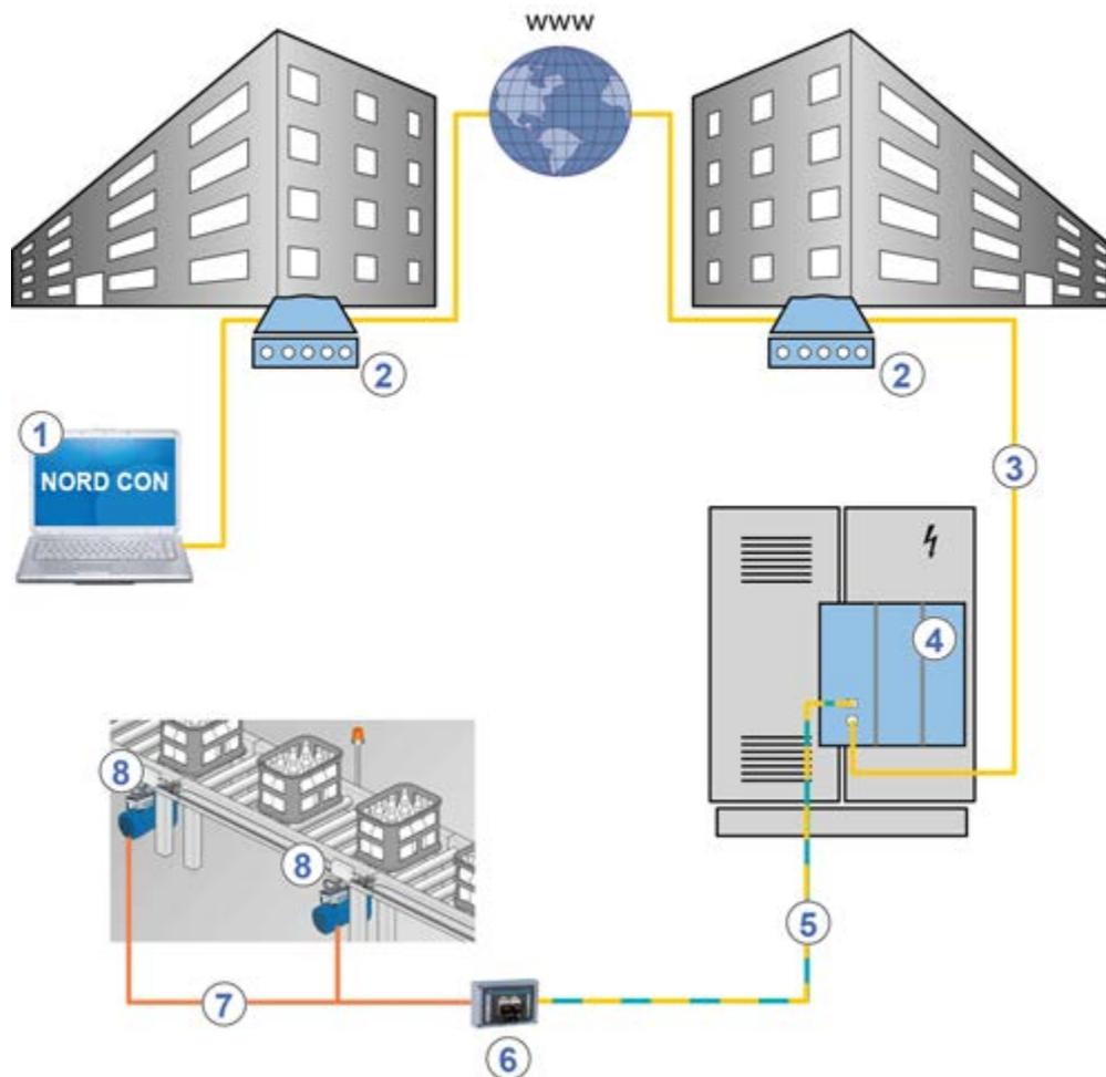
Figure 9: Remote maintenance via Internet (schematic diagram)
