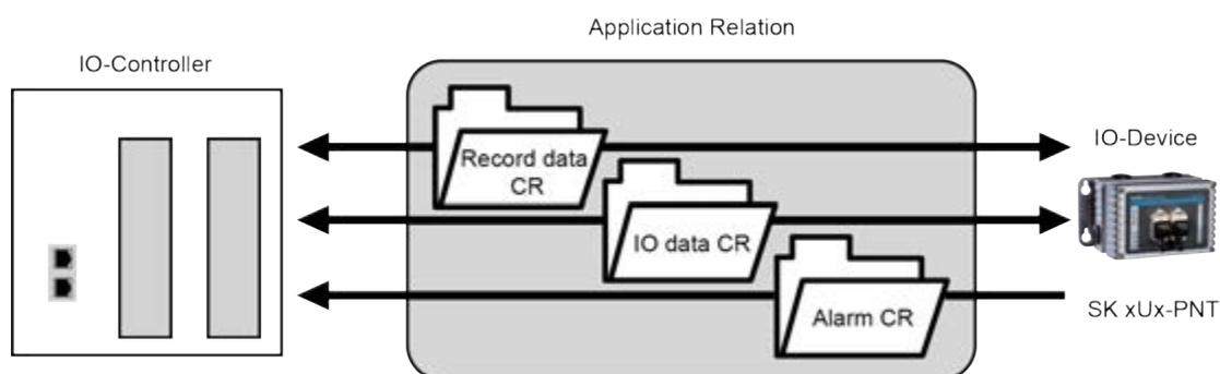
Figure 1: PROFINET IO communication via Application Relation AR
