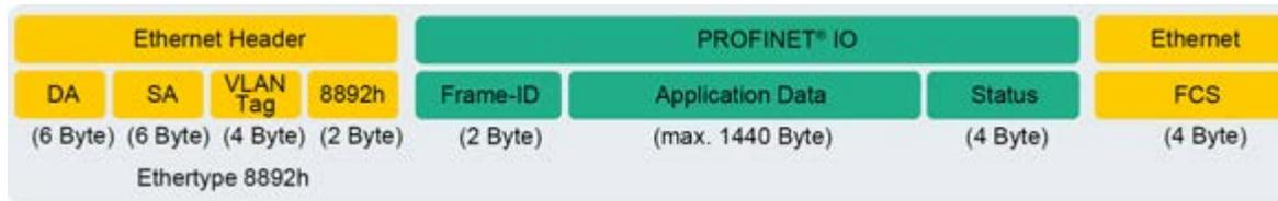
Figure 6: PROFINET IO telegram (communication within a sub-net)
