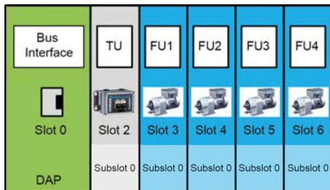
Figure 11: Example – PROFINET IP device model for decentralised devices
