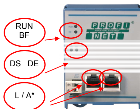
Fig. 4 Location and designation of the LEDs
