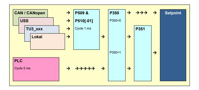
If the PLC is activated (P350=1) preselection of setpoints from external sources (main setpoints) is carried out via P509 and P510[-01] Via P351, a final decision is made as to which setpoints from the PLC or values input via P509/P510[-01] are used. A mixture of both is also possible. No changes to the auxiliary setpoints (P510[-02]) are associated with the PLC function. All auxiliary setpoint sources and the PLC transfer their auxiliary setpoint to the frequency inverter with equal priority.
