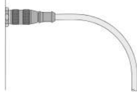
Freely laid cable
