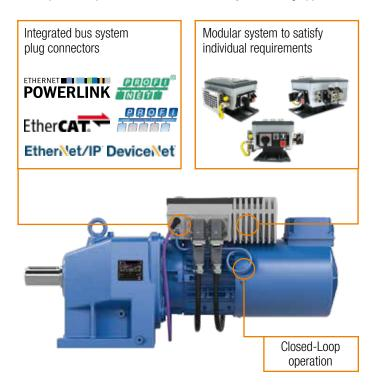
In this decentralized drive setup, signal interference is not an issue and long distances with screened cables are not required. The drives have safety functions on board and ensure direct communication between encoder and inverter (Closed-loop operation). Additionally plug-and-work power and bus system connectors greatly simplify installation and maintenance. This saves time and expenses.
