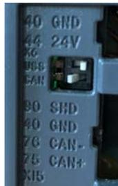
Figure 6: Terminating resistor setting
