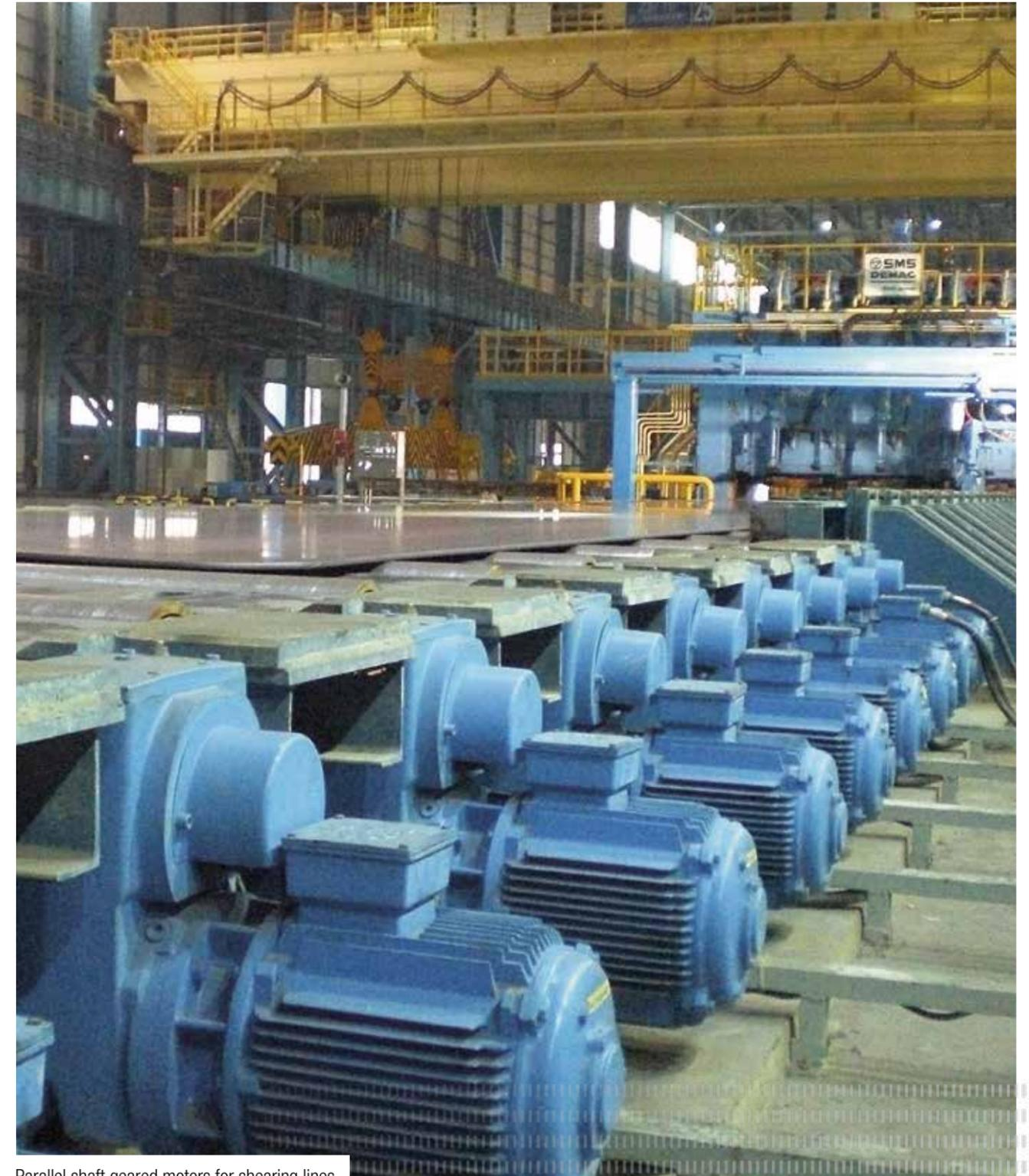
Parallel shaft geared motors for shearing lines
