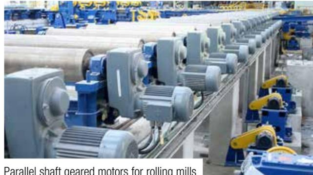
Parallel shaft geared motors for rolling mills
