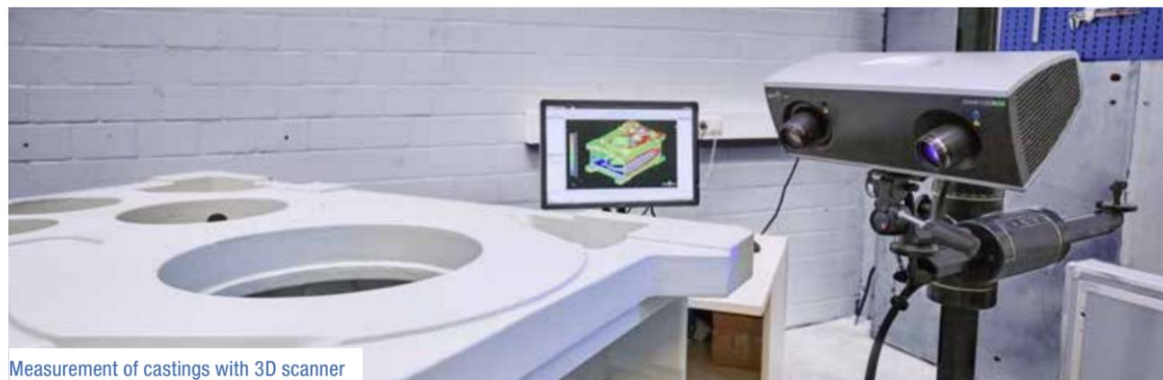
Measurement of castings with 3D scanner
