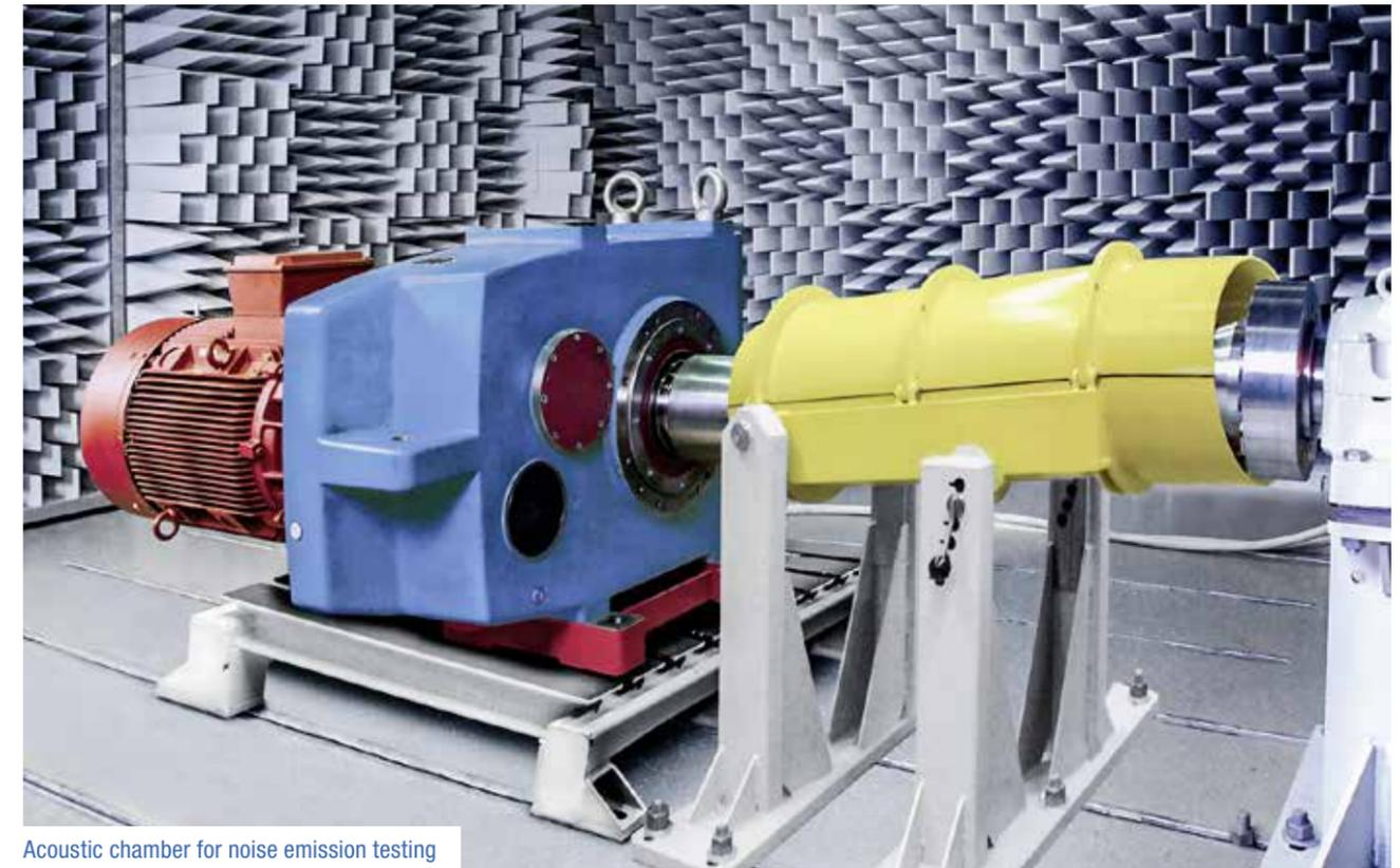
Acoustic chamber for noise emission testing
