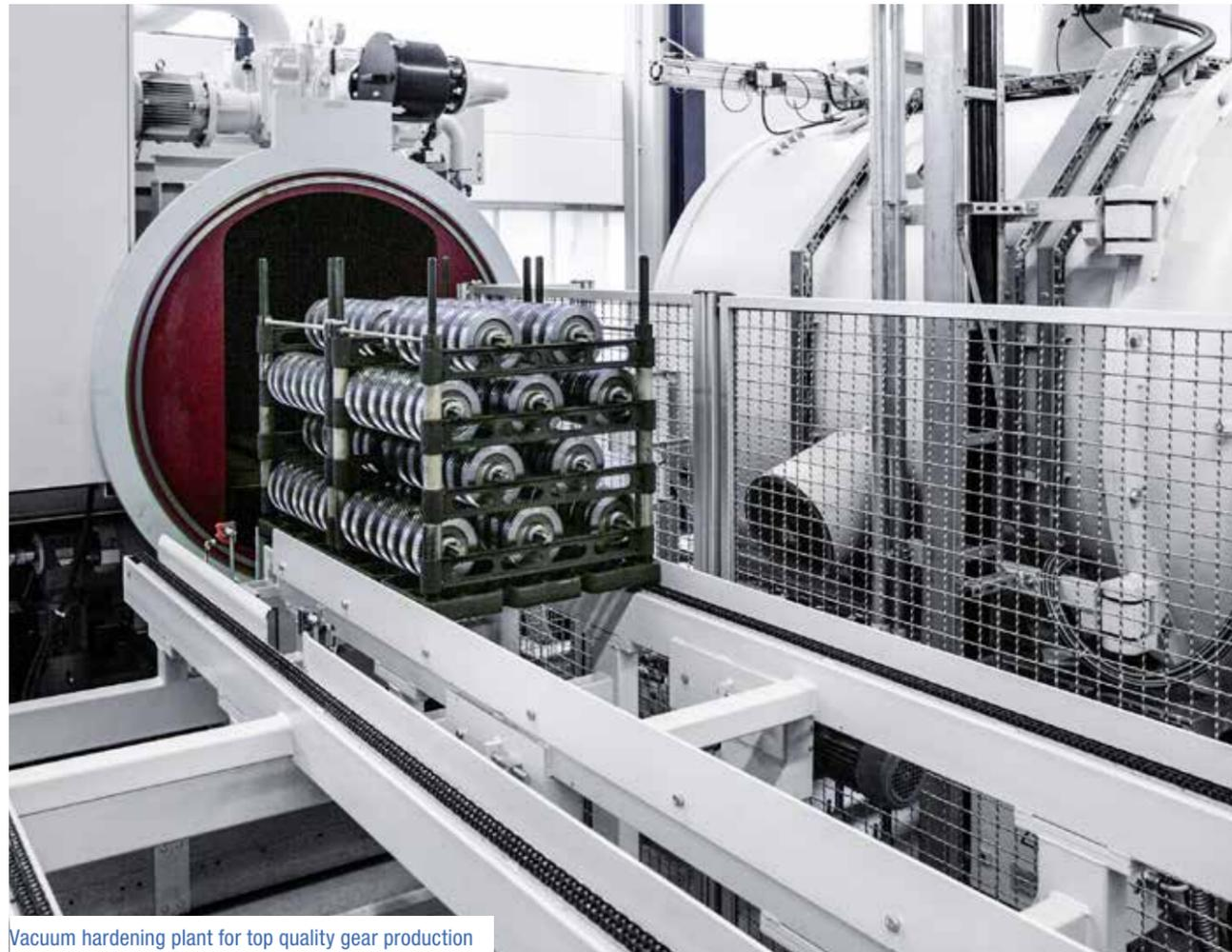
Vacuum hardening plant for top quality gear production
